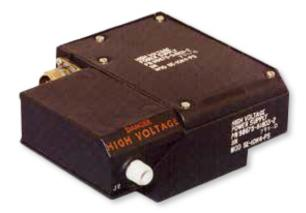
Espey developed this power supply for the AN/APN-169 station-keeping radar system for a prime military contractor program. This multiple output, 10 kV, high voltage DC-DC converter module is designed for extreme airborne environmental conditions.
