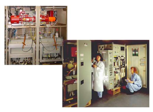
Espey developed this, solid state, high voltage power supply, as the major subsystem of a 150 kW, 8.8% duty cycle, coherent S-Band TWT radar transmitter system. The solid state 45 KV DC power supply is rated at 60 kW average output power at 19 amps peak for pulse widths from 8 to 300 microseconds.
